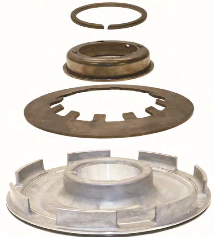
PISTON ASSEMBLY WITH ONE-WAY CLUTCH
