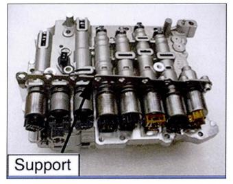
19. Refer to the DTC recorded in Step 1 and replace the related solenoid
